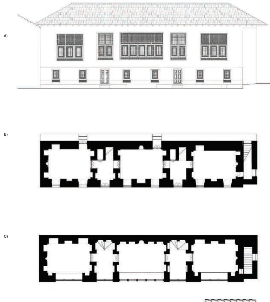
Figure 37. Drawings of the Shekikhanov's House a. Main facade b. Ground floor's plan c. First floor's plan
